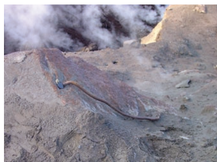
Two GPS stations were destroyed as a result of the recent eruptions. AV05 stopped reporting data in mid-January. Above are the remains of this Augustine GPS station without a trace of the hut, solar panels, or batteries. Image courtesy of USGS.
