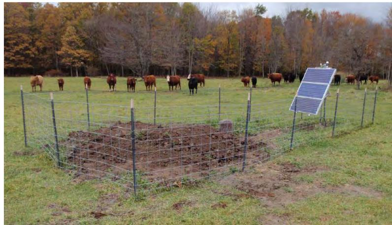
A completed seismic station has a small footprint with just a fence surrounding the solar panels and a mound of dirt covering the vault. The vault contains the seismometer, batteries, and electronics. Pictured here is station K50A in Casco, Michigan, where fencing is essential for keeping out the landowner's curious cows.
