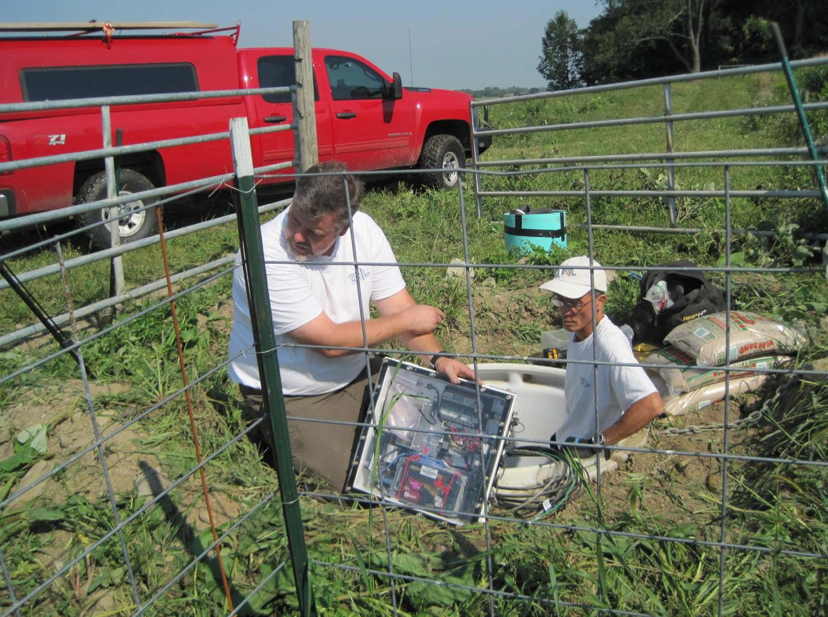
Station specialists Mike Couch and Doan Nguyen get ready to install the vault interface enclosure for station K57A, which contains the electronics equipment that controls the station's power, data collection, and communications. *Photo credit: Perle Dorr*
