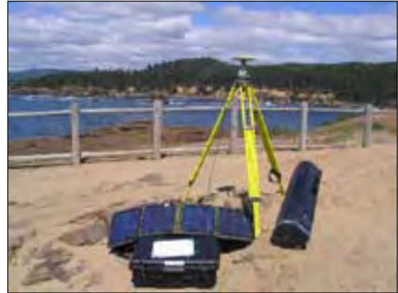
The first deployment of the EarthScope GPS Campaign Systems occurred along the Oregon coast in the summer of 2005.
