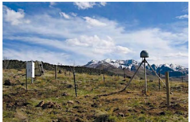
Figure 1.5. Completed GPS station near Delta Utah and the Wasatch Fault Zone. DDBM with radome housing GPS antenna is on the right. Enclosure housing GPS receiver and cellular modem is on the left. Security fence prevents equipment damage by livestock.
