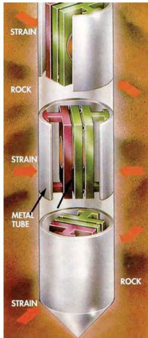
Figure 1.8. Schematic representation of a GTSM tensor strainmeter. The two green plates are a fixed distance apart. The red plate moves relative to the green plates as the borehole deforms.
