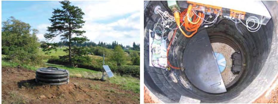
Figure 2.3. A typical Transportable Array station showing the relationship of the equipment inside the enclosure and the solar panel.
