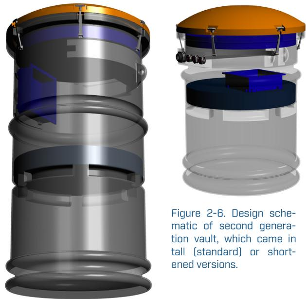
Figure 2-6. Design schematic of second generation vault, which came in tall (standard) or shortened versions.
