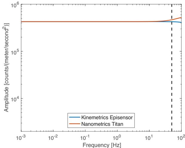
Figure 2-17. Individual responses of the two strong motion accelerometers operated by the TA. Dashed line indicates the Nyquist frequency.
