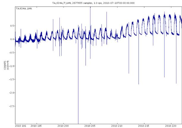
Figure 3-24. Continuous time series from 7/10/2010 to 8/10/2010 (31 days) at TA.634A..LHN. The diurnal signal relates to varying temperature of the vault throughout the day. The variations in amplitude on the time series relate to the magnitude of the temperature change experienced inside the vault.
