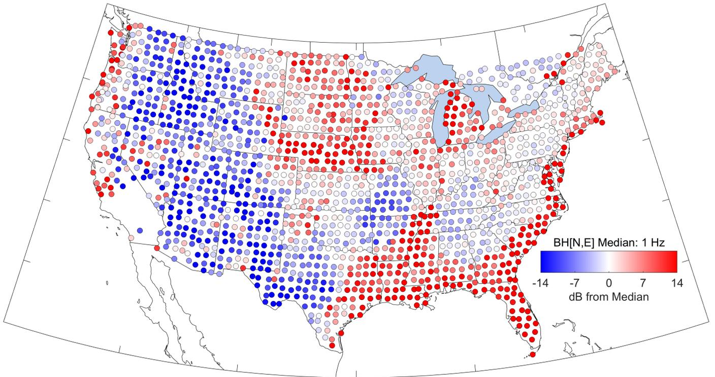
Figure 3-13. Deviation from the median of the median noise spectra at -1 Hz/1 sec.
