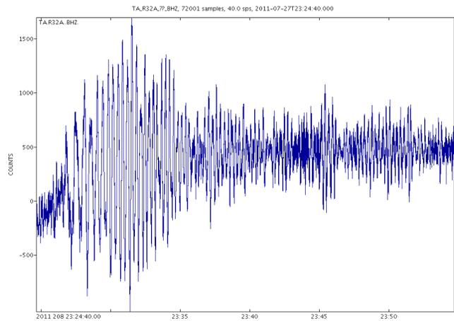
Figure 3-19. The effect of the recentering is shown on the time series for TA.R32A..BHZ. The recentering and subsequent settling of the instrument is displayed for five minutes and then an additional 30 minutes at different vertical scales.
