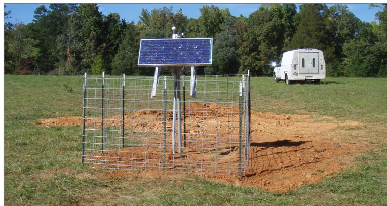
Figure 2-10. TA.KMSC had excellent skyview, and with cellular telemetry it only required a single solar panel to operate.
