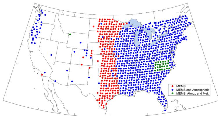
Figure 2-19. Distribution of auxiliary atmospheric and meteorological sensors across the TA: red = MEMS only, blue = MEMS/barometer/infrasound, green = MEMS/barometer/infrasound/meteorological packages.
