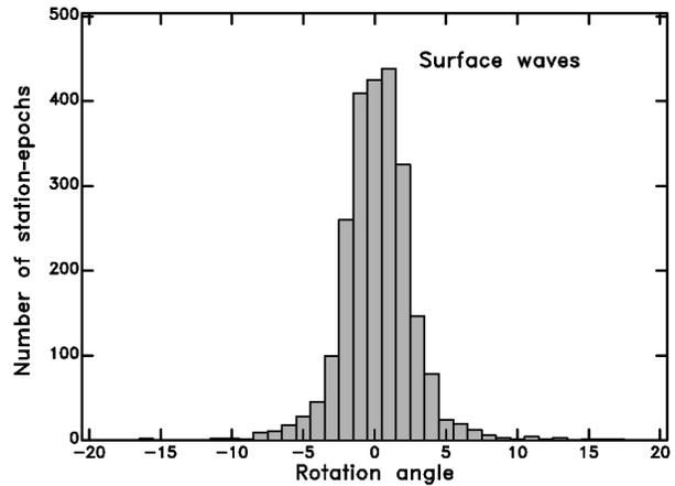
Figure 2-22. Histogram showing the distribution of robust median rotation angles for 2365 station-response epochs based on analysis of orientation using teleseismic surface-wave (Ekström and Nettles, 2018).
