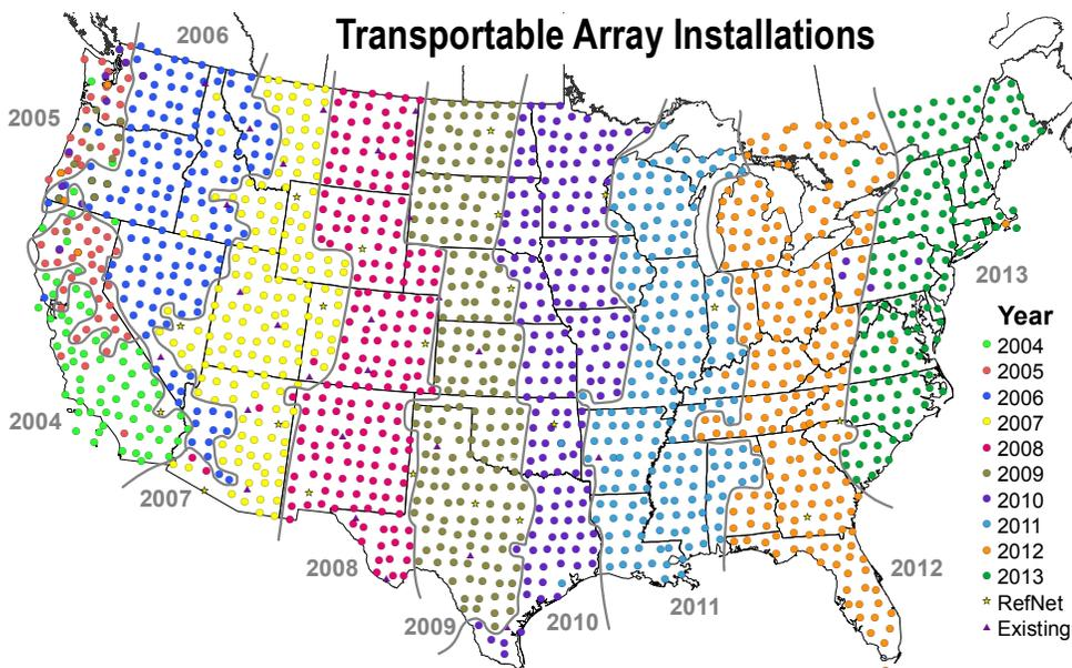
Figure 1-3. Map of the 10-year TA as built. The final station locations achieved the planned grid, year-by-year progress followed the initial plan closely, and additional stations were sited in Canada.
