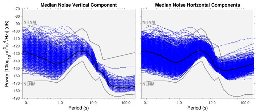
Figure 3-10. The median spectra (blue) of the vertical (left) and averaged horizontal (right) components for each TA station, with the median (black) of all stations and the NHHM/NLNM (gray).
