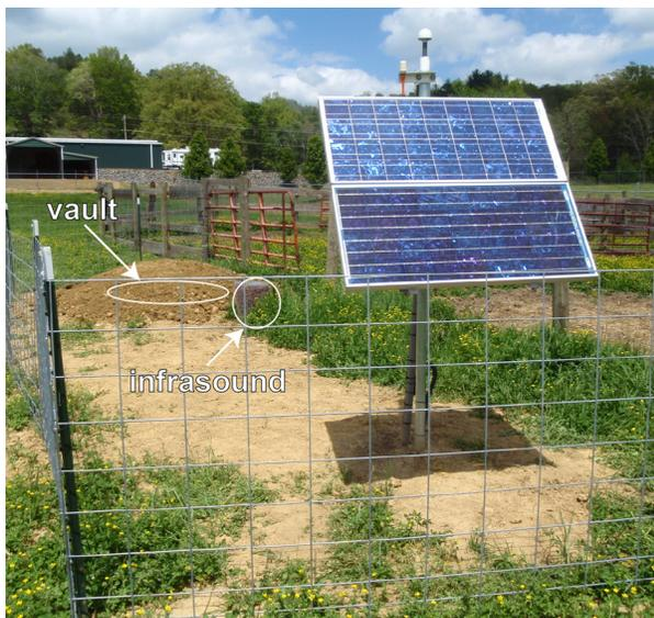
Figure 1-1. TA.W52A (Murphy, NC) represents the finalized design of a TA seismic station, with solar panel assembly adjacent to an infrasound sensor cage and buried seismometer vault.
