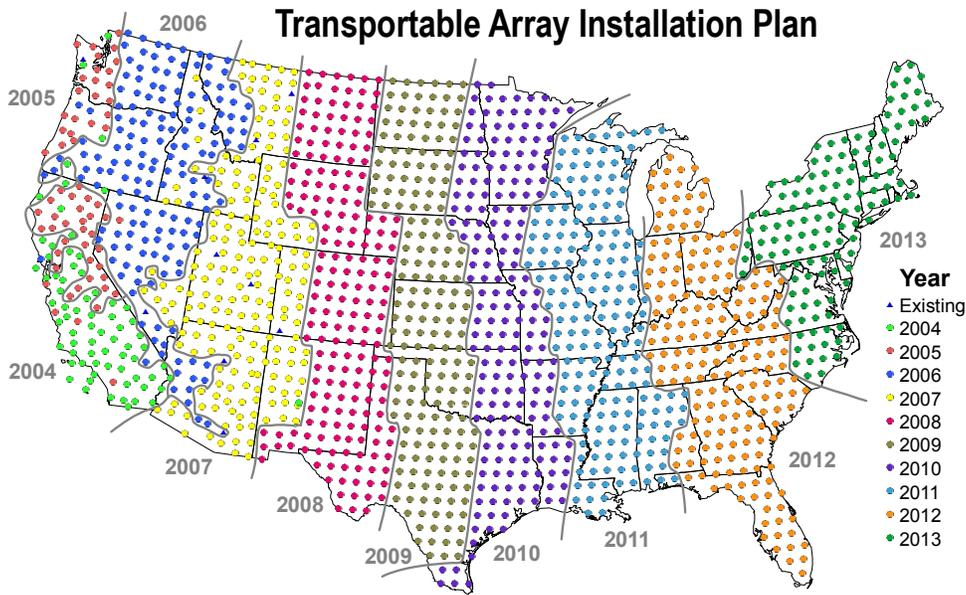
Figure 1-2. Map of the 10-year deployment plan for the TA, showing the nominal grid spacing of 70 km between stations and illustrating the planned year-by-year deployment progress. Note: The westernmost stations reflect the actual deployment locations.
