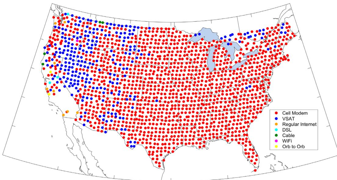
Figure 2-25. Final telemetry configuration for TA stations, through 7/20/17.
