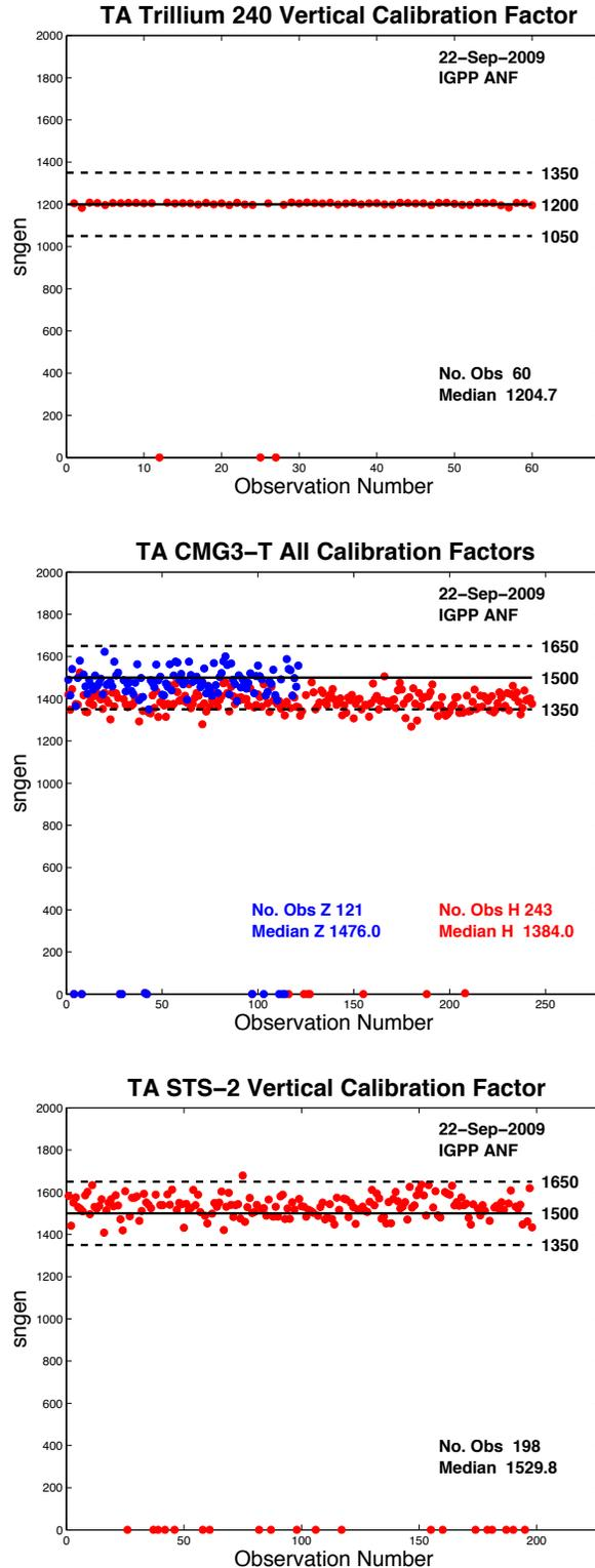
Figure 3-17. Calibration factor [sngen] plots for various instruments and components show the spread of results within reasonable bounds.
