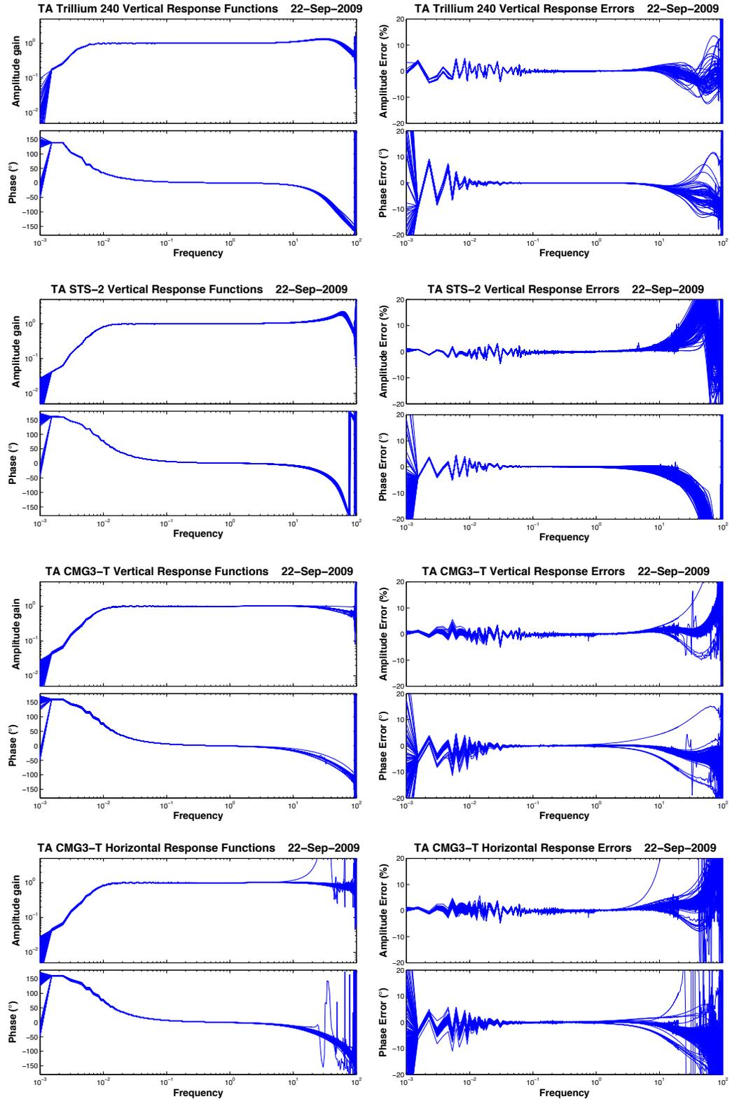
Figure 3-16. Amplitude and phase response functions for each type of TA seismometer (left) and errors in percentage relative to the nominal response (right). Both the raw measurements as well as calculated error for amplitude and phase reflect that most TA seismometers operated consistently with a nominal response function.
