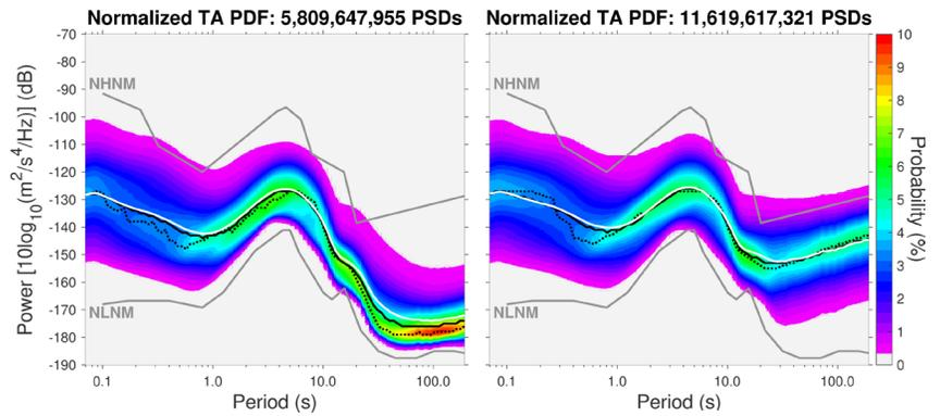
Figure 3-9. Composite probability density function of all power spectral density measurements from the TA network for vertical (left) and combined horizontal components (right). The mean (white), median (black), and mode (dotted black) of all spectra are displayed along with the NLNM and NHHM. The y-axis (power, dB) has logarithmic units; therefore, increments relate to an increase or decrease in power by a factor of 10.
