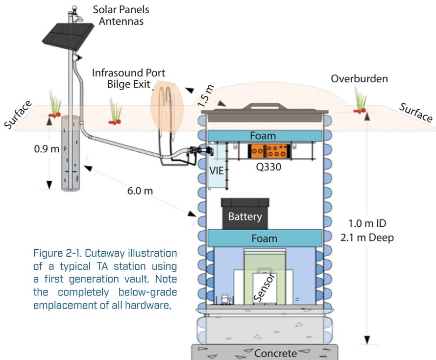
Figure 2-1. Cutaway illustration of a typical TA station using a first generation vault. Note the completely below-grade emplacement of all hardware,
