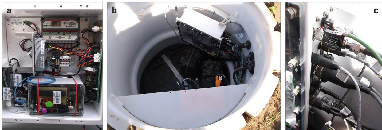
Figure 2-8. Close-up of the vault interface enclosure, or VIE: (a) internal components with lid removed, (b) as installed in a typical vertical configuration (TA.L62A), and (c) the connections on the side of each unit (TA.D60A).
