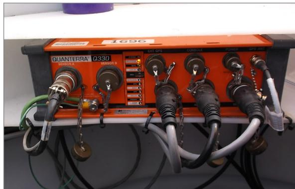
Figure 2-24. Typical Q330 installation at TA.D56A.
