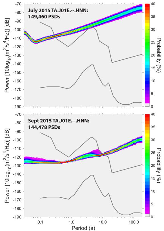
Figure 2-18. Example of the effect of “zinc whiskers” in monthly power spectral density estimates, before and after replacement of the sensor.
