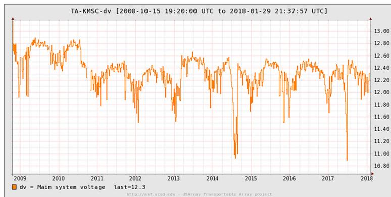
Figure 2-9. Voltage levels at TA.KMSC (a RefNet station that did not use grid-based naming scheme) show seasonal variations in power levels based on constant discharge and variable input voltage from its solar panel.
