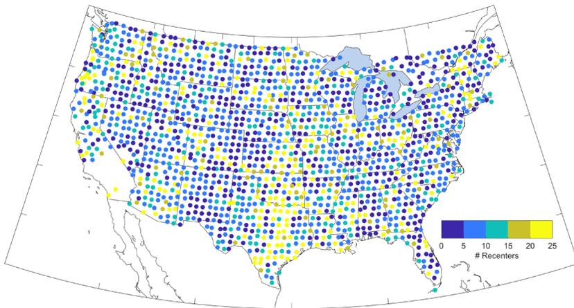
Figure 3-20. Mass recenterers at each TA station through 7/20/17. Color scale saturates at 25.
