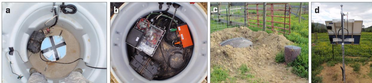
Figure 2-7. TA.W52A (Murphy, NC), featuring (a) completed lower chamber, with seismometer wrapped in blue foam insulation and battery to its left, (b) completed upper chamber, (c) buried vault with infrasound enclosure, and (d) solar/gps/communications mast. Note that this is a shorter version of the second generation vault, with the VIE resting horizontally.
