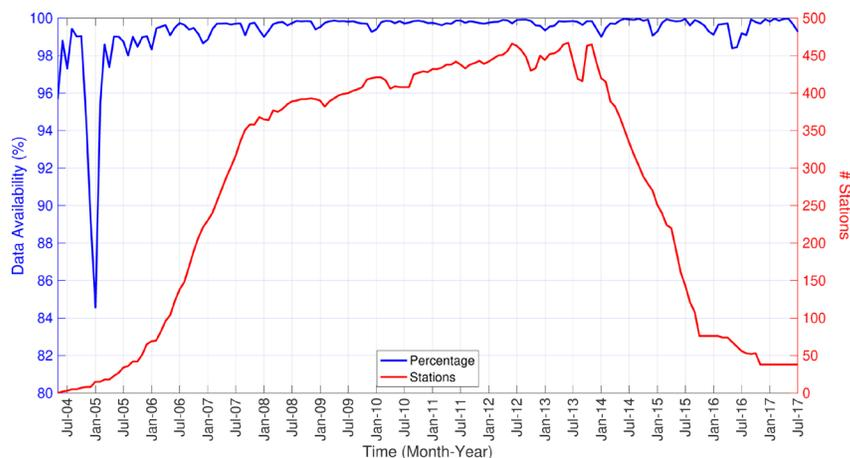
Figure 3-2. Comparison of average data availability and number of deployed stations for the TA per month.
