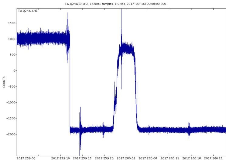
Figure 3-22. “Half amplitude” behavior observed for TA.Q24A..LHZ. The time series shows the characteristic sudden amplitude reduction and large offsets which cannot be linked to ground motion.
