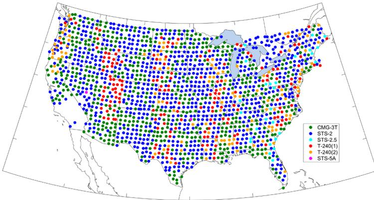
Figure 2-13. Distribution of seismometer types operated across the TA network, based on the initial broadband seismometer installed at each station.
