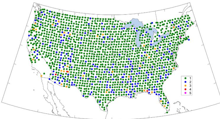
Figure 2-15. Count of broadband seismometers installed at each TA station.
