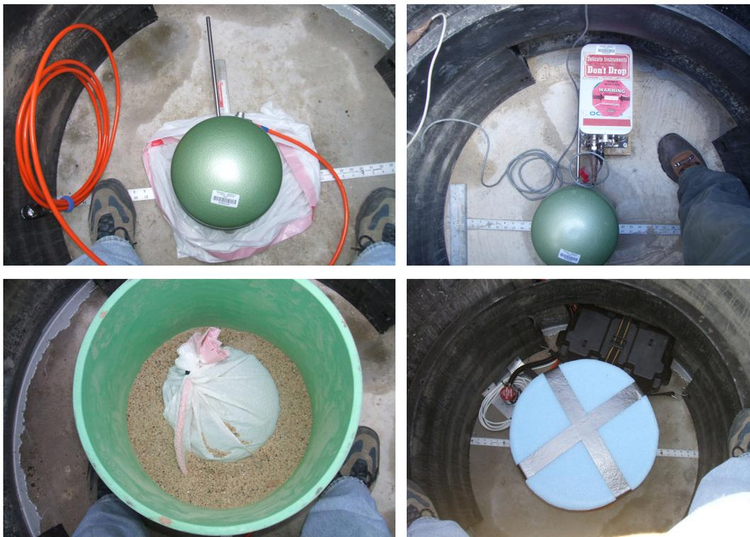
Figure 2-21. Example of orienting an STS-2 seismometer using the Octans at TA.N15A. Notice the shock watch stickers that might indicate an Octans had suffered a crippling impact. Once oriented, the sensor is then packaged and insulated.
