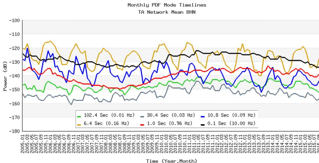
Figure 3-11. Mode of the cumulative spectral power of the entire TA for six different periods of interest. This analysis was automated and produced regularly by the DMC for each station-channel to monitor network performance.
