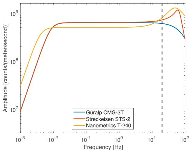
Figure 2-14. Individual responses of the main three broadband seismometers operated by the TA. Dashed line indicates the Nyquist frequency.
