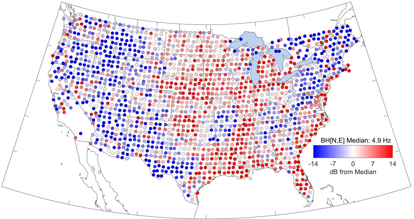
Figure 3-12. Deviation from the cumulative median for the network of the median noise spectra at ~4.9 Hz for the vertical and averaged horizontal components. Color scale limits are based on the approximate 10<sup>th</sup> and 90<sup>th</sup> percentile distribution of measurements.
