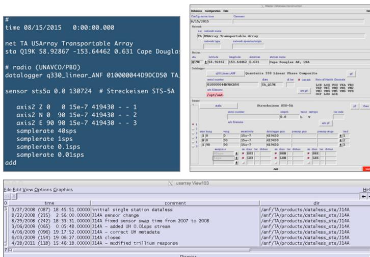
Figure 4-10. Example from batch file input for dbbuild metadata generation (top left), GUI interface to dbbuild (top right), and view of database table that tracked metadata updates (bottom).
