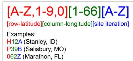
Figure 2-3. Definition of a TA station code, with examples.
