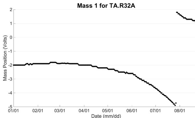
Figure 3-18. An episode of mass position drift and recentering for TA.R32A, which operated an STS-2 with limits of  $\pm 12$  V.
