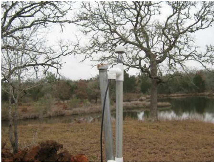
26. Install GPS antenna using reducer bushing and nipple
