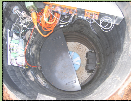
View into vault. Sensor encased in sand, Q330 and baler on shelf, foam insulation
