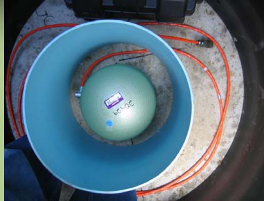
Sensor alignment. Leveling and insulation takes over an hour
