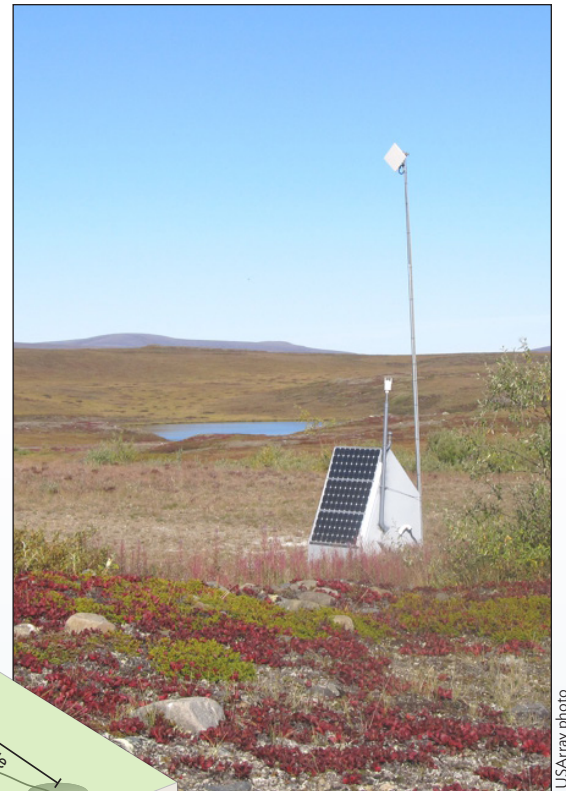
The photo and diagram above demonstrate a new station design created specifically for Alaska. Located at Toolik Field Station, the site combines basics of the Transportable Array's Lower 48 station design, with attributes used in the existing seismic monitoring network in state. Specific attention to weather conditions, sunlight and wildlife are included in the new design.
