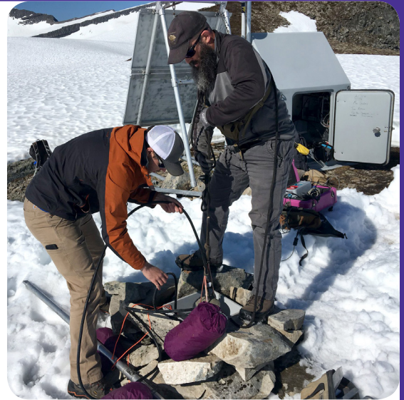
Alaska Transportable Array Station Specialist Jeremy Miner (right) and AEC Seismic Network Technician Evan McArthur (left) install a new seismometer at station O20K on Slope Mountain located southwest of Anchorage and on the western side of Cook Inlet. This station has been transitioned to the AEC for long-term operation. Photo: Tim Dittmann, UNAVCO
