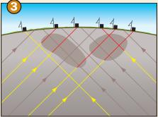
Six seismometers catch enough recorded waves for scientists to start determining the borders of the structures. With dozens of seismometers, scientists can produce an image of a slice of the Earth.
