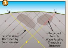
1 Two seismometers on the surface record incoming seismic waves. Only one recorded wave passes through part of one of the structures with different properties than the surrounding material. Scientists examining the recorded seismograms would infer that only one structure is present instead of two.
